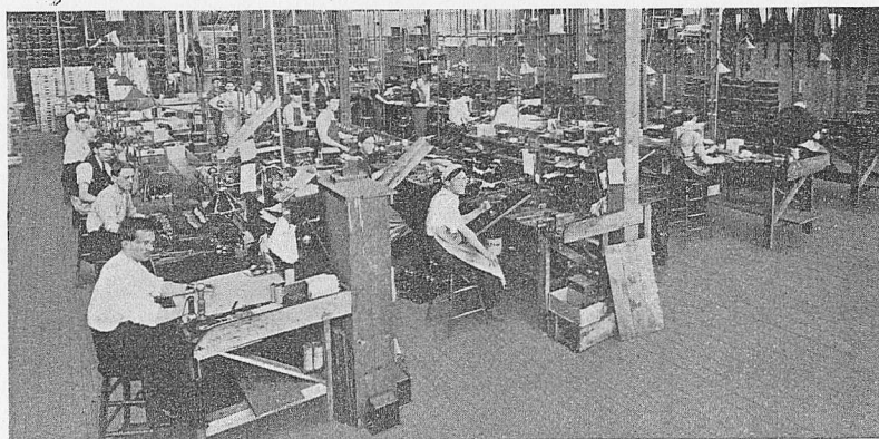
Fig. 29.—Assembling and Adjusting Receivers.
