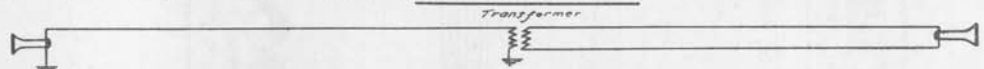
Method of connecting single [earthed circuit] Line to Metallic Line by means of Transformer
