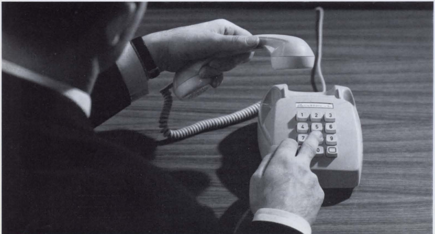
Fig. 13 Pushbutton telephone used with Pentaconta exchanges
